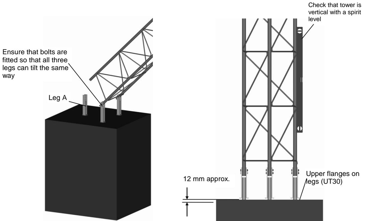
To tilt the tower, remove both bolts from leg A. (see above). Remove the lower bolts and loosen the upper bolts in the other two legs.
