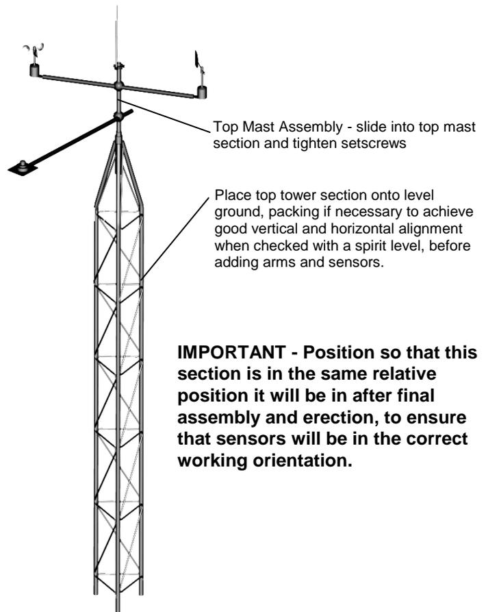
Figure 2-2 Top Tower Section at Ground Level
