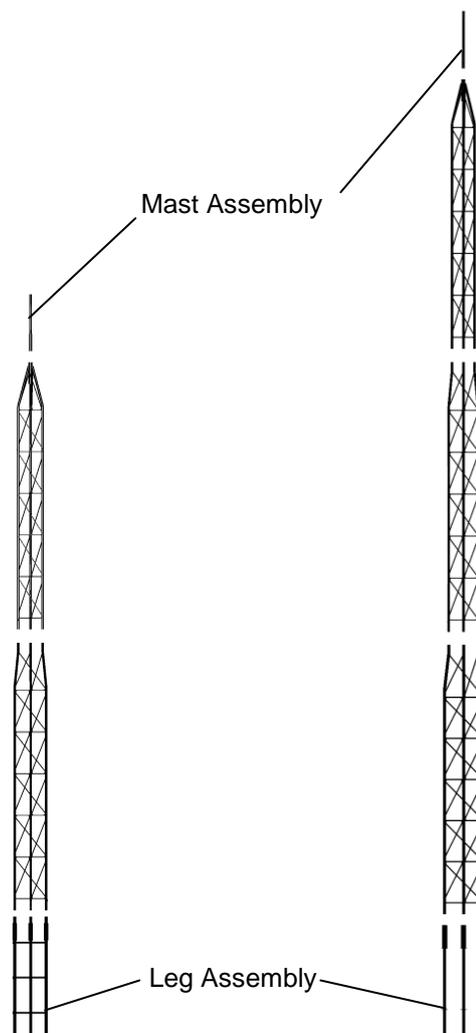
Figure 1-1 UT20 and UT30 Towers, showing Tower Sections
