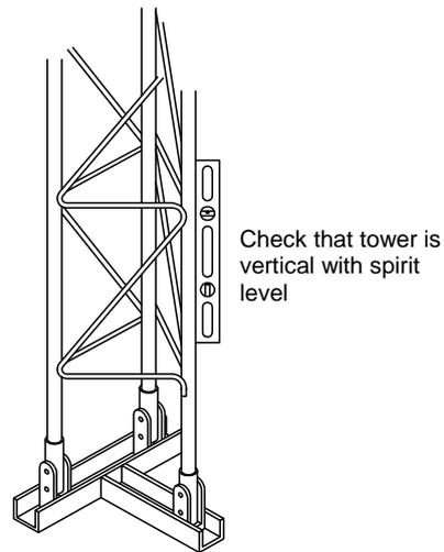
Figure 1-4 Special Roof-Mounting Base Installation for UT30
