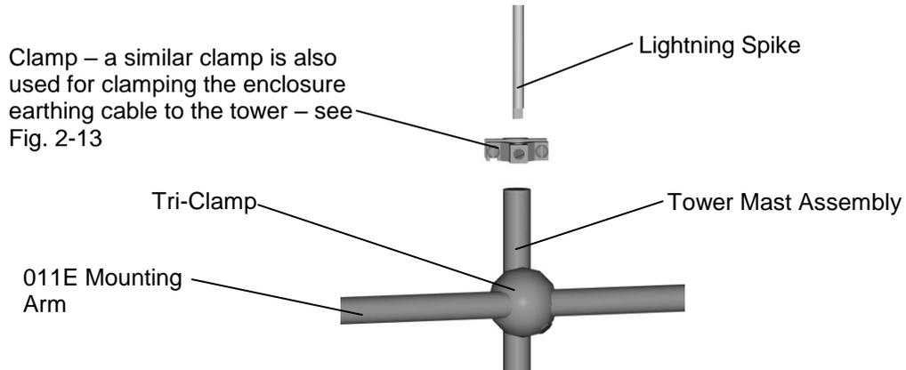
Figure 2-1 Attaching the Lightning Spike
