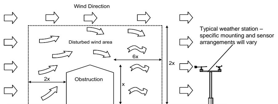
Figure I-1 Effect of Structure on Air Flow
